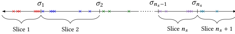
Fig. 1. Partitioning the spectrum of interest into several slices or subintervals which may be computed simultaneously.
